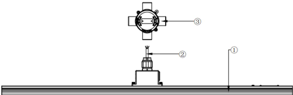
1. For luminaire model with suffix "WHT": Insert the cord (2) through the conduit (not shown, provide in the field) into the Junction Box (3) (provide in the field).
