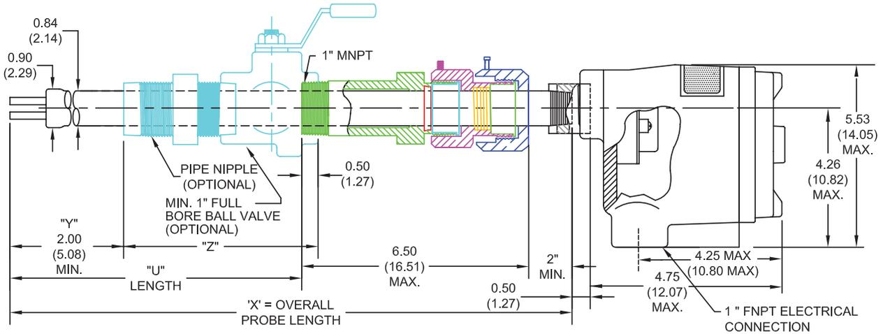
CLASSIC® 816 Retractable Packing Gland Threaded - 1" MNPT - c/w Retaining Chain - to 125 psi
