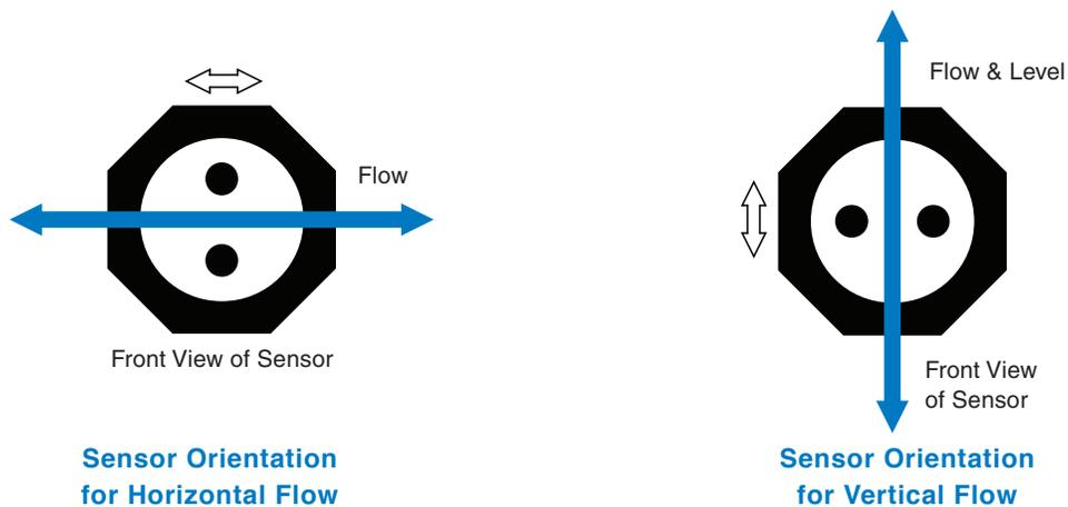
**Guidelines for Flow Applications - Liquids, Slurries, Air, Gas**
