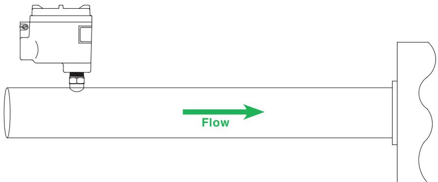
**Note:** Flow profiles will tend to be smoother as the downstream distance between the bend, elbow, valve, pump, fan or compressor and the switch increases.
