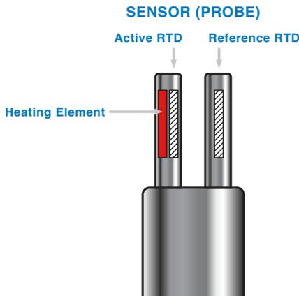
Kayden thermal switches use proven thermal dispersion technology to create a very accurate, economical and rugged device for sensing flow, point level, liquids interface and temperature.
