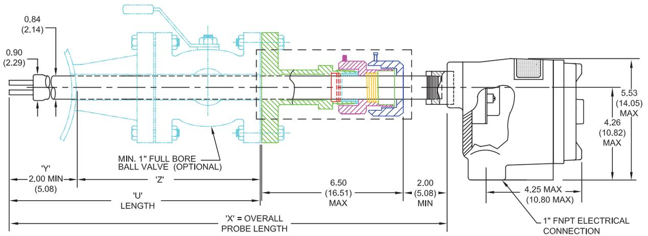
**CLASSIC® 814 Retractable Packing Gland Flanged - 1" MNPT - c/w Retaining Chain - to 125 psi**
