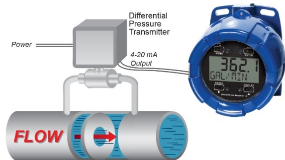
PD6820 Displaying Flow Rate by Extracting Square Root from DP Transmitter Signal.
