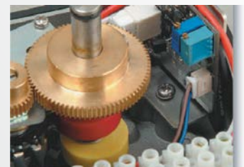
Position Transmitter 12.5VDC to 37VDC, 4-20mA (Excludes APL-2)
