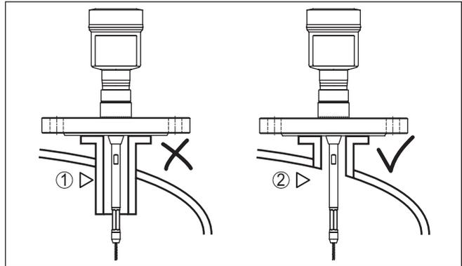
Fig. 5: Montar as luvas de forma nivelada
