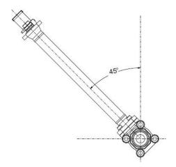
2.1.2.As the cryogenic valve is unidirectional, it is required to make sure the direction of the arrow mark on the body match the flow of the pipeline when installing the valve. The vented hole of the ball will be upstream when the valve is closed.
