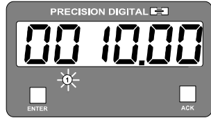
Meter displaying preset offset between set points 1 and 2
