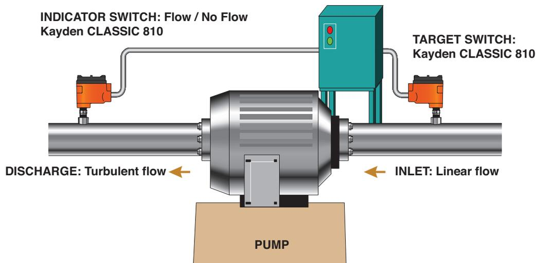
**Figure 1 - Kayden Classic used in pump protection / monitoring**
