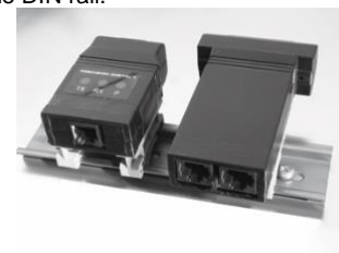
Figure 8. Typical Installation of DIN Rail Mounted Devices
