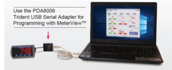
Note: Trident meter is not powered from USB connection and requires external power to be programmed.
